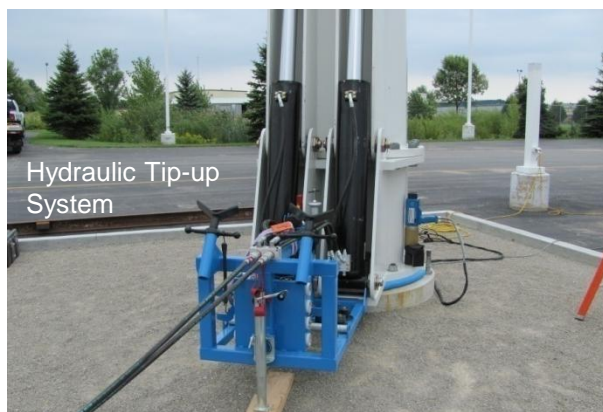
Approximately 8 to 10 minutes to raise or lower the VP-20
