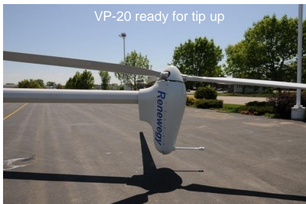
Approximately 8 to 10 minutes to raise or lower the VP-20
